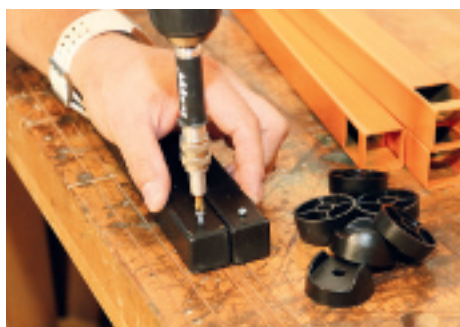
▲ Small self-tapping screws set the rack support positions
