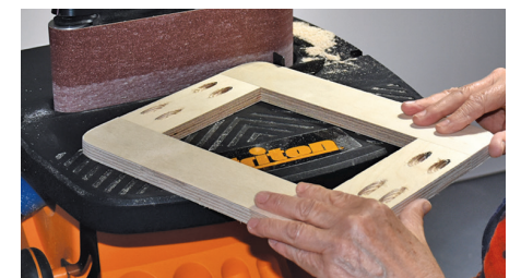
Sanding the frame corners on a Triton bench-top sander
