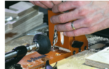
Using a 10p piece to set the correct drill depth
