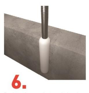
Push and turn the treaded rod or rebar into the hole containing the Soudafix chemical anchor resin.
