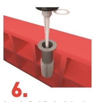
Apply the Soudafix chemical anchor resin into the sleeve in the drill hole, ensuring the resin is mixing properly before application.
