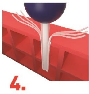
Clean the hole using a blow-out bulb, pump or compressed air (4x).
