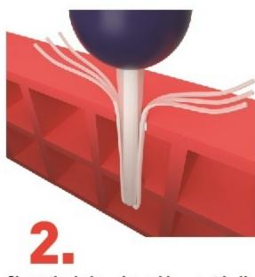
Clean the hole using a blow-out bulb, pump or compressed air (4x).
