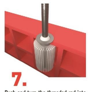
Push and turn the threaded rod into the hole containing the Soudafix chemical anchor resin.
