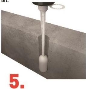
Apply the Soudafix chemical anchor resin into the drill hole, ensuring the resin is mixing properly before application.
