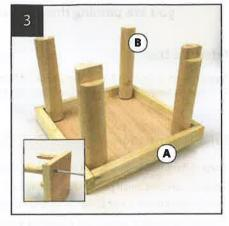
Repeat steps 1 and 2 until 4x (B) support are attached to each corner of (A) base.
