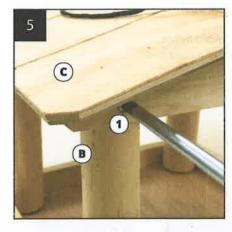
Secure the Roof (C) in place by inserting a (1) screw through (C) into (B) on each support.
