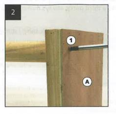
Attach 1x (B) to (A) as shown above using 1x (1).
