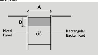
**Dimension A** - Joint Width **Dimension B** - Sealant Depth and Bond Surface
