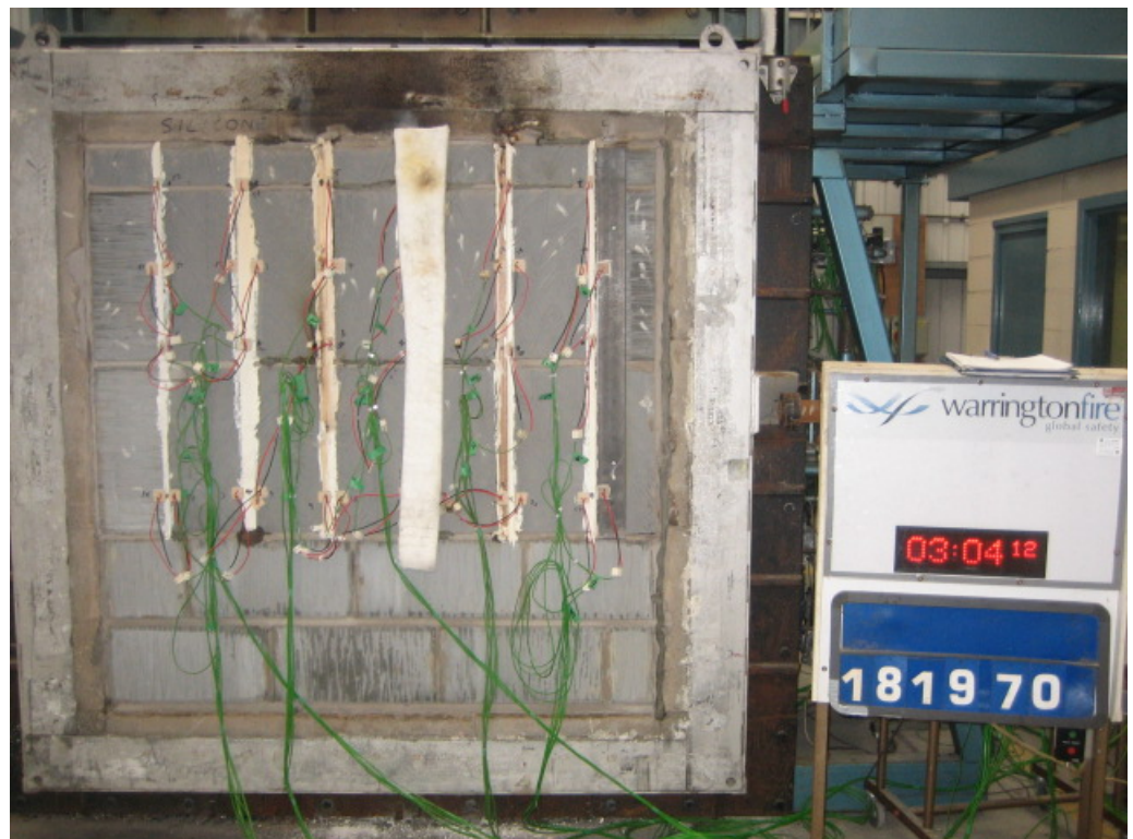
The unexposed face of the wall construction after 184 minutes of testing
