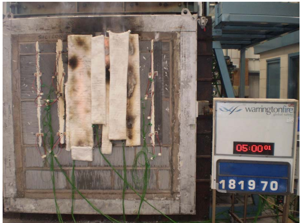
The unexposed face of the wall construction after 300 minutes of testing
