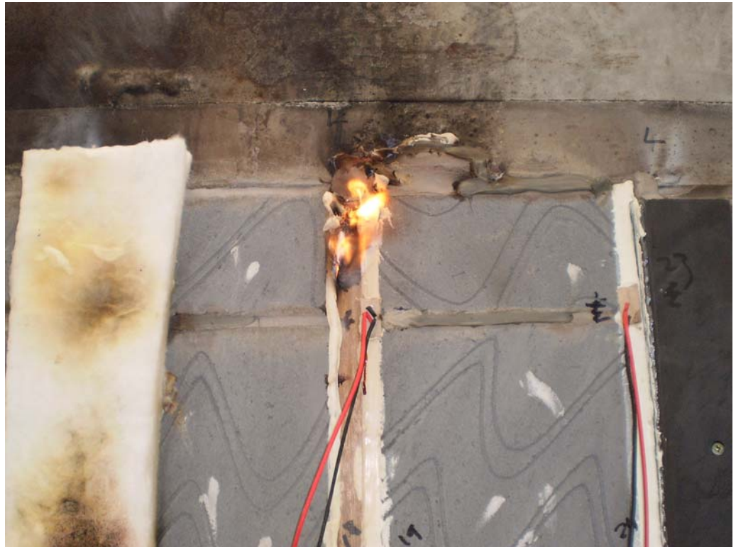
Integrity failure of Specimen K after 208 minutes of testing
