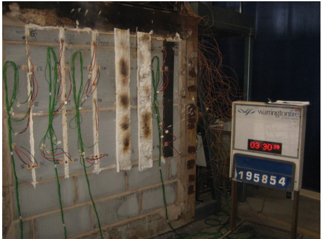
The unexposed face of the wall construction after 210 minutes of testing
