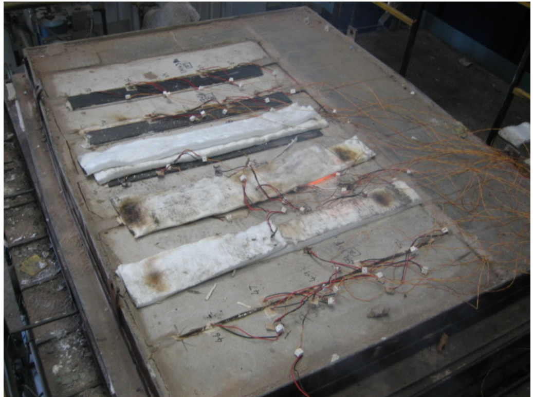
The unexposed face of the floor construction during the test
