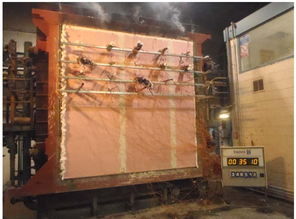
The unexposed face of the specimens after a test duration of 35 minutes
