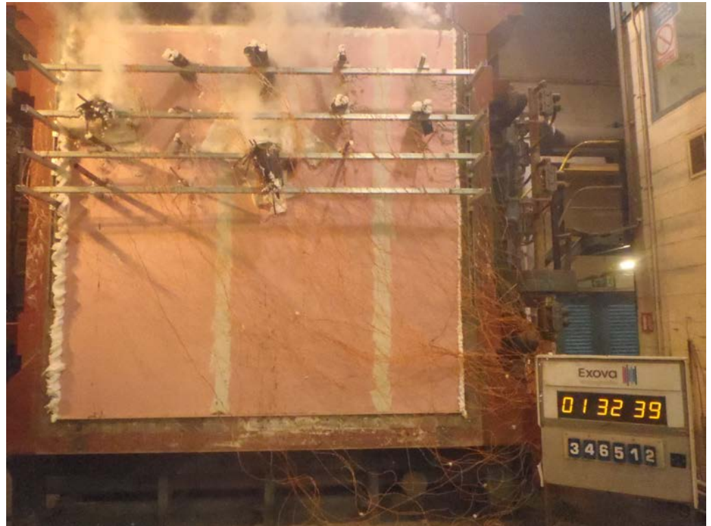
The unexposed face of the specimens after a test duration of 92 minutes
