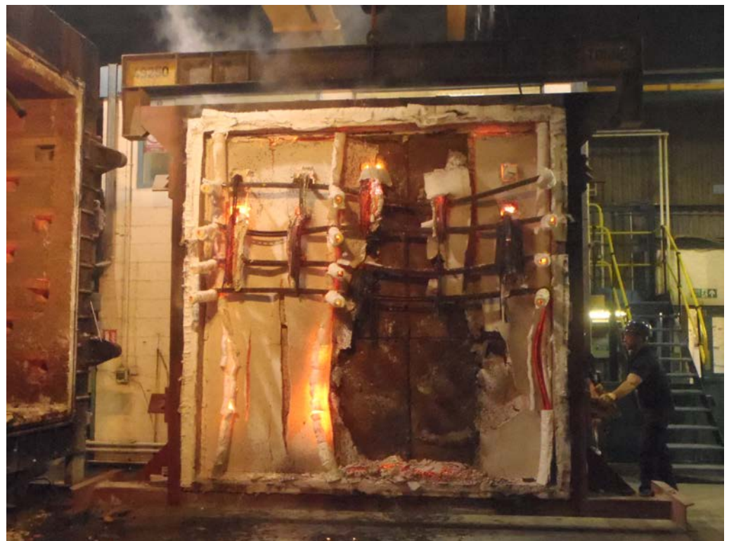
The exposed face of the specimens immediately after the test
