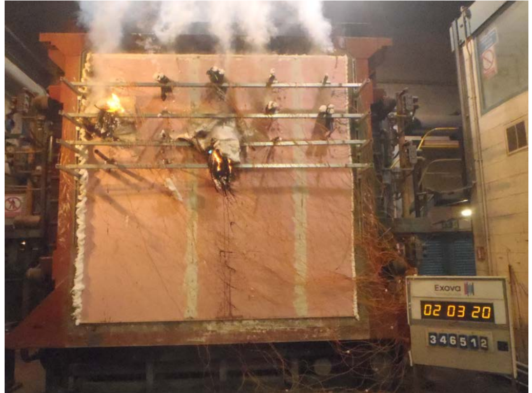
The unexposed face of the specimens after a test duration of 123 minutes
