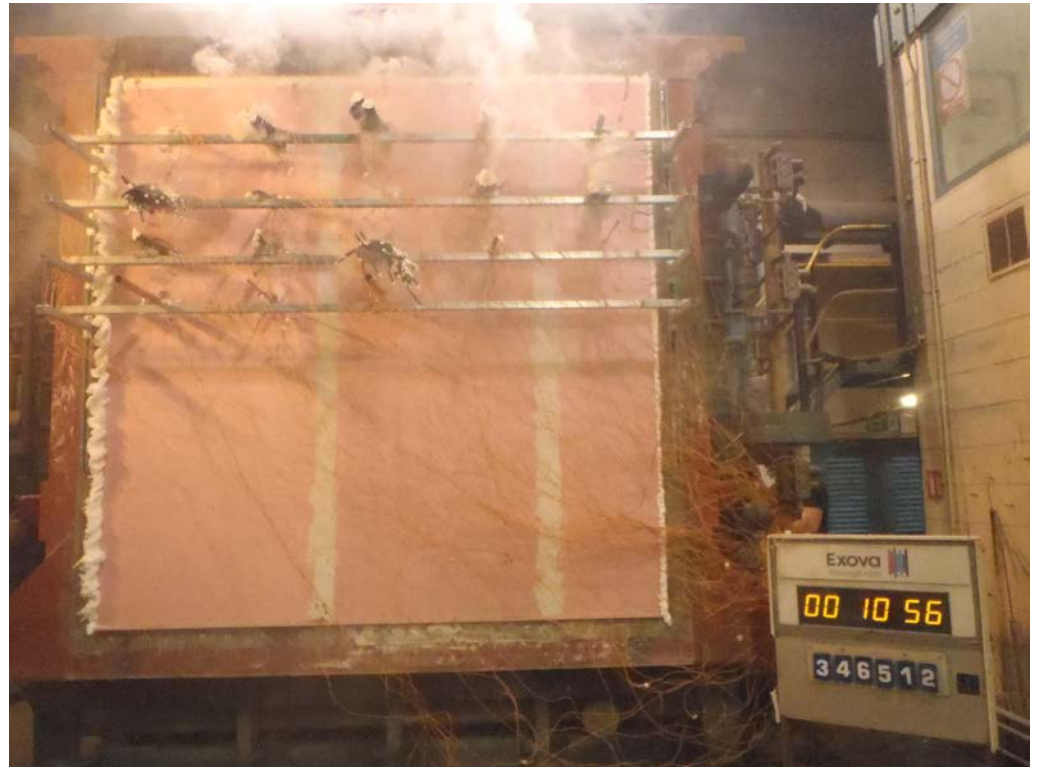
The unexposed face of the specimens after a test duration of 10 minutes
