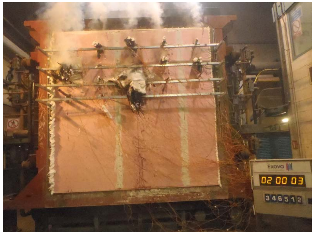
The unexposed face of the specimens after a test duration of 120 minutes
