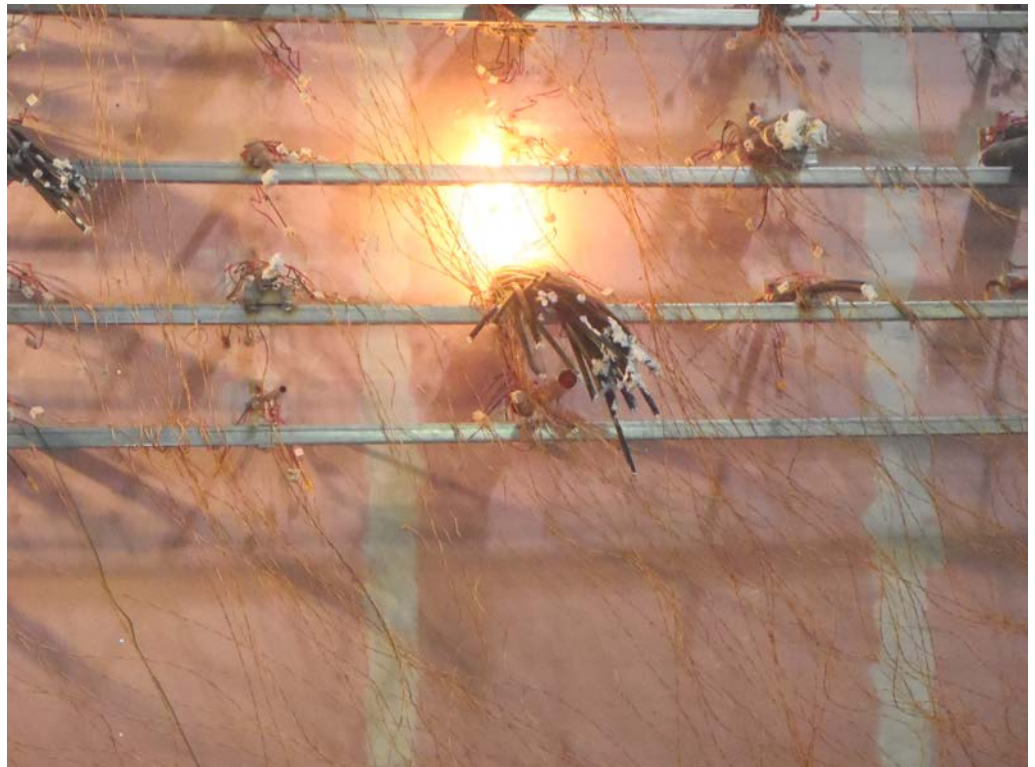
Integrity failure of Specimen M after a test duration of 60 minutes
