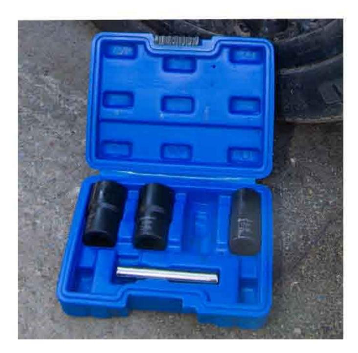
1 Find the suitable socket to fit the outer diameter of your locking wheel nut.
