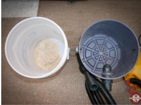
The filter is located in the lid. The vacuum/collection bucket assembly is ready to be used.
